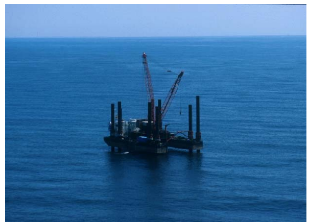
Figure 5-4: Drilling and conic penetration test with a platform from Mohiba.
