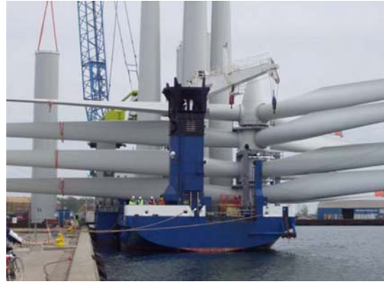
Rack for stacking four rotors; source: Siemens Wind Power 69
